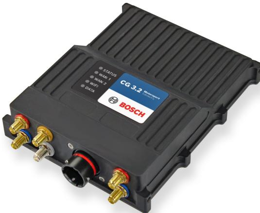
The CG 3.2 is the new Bosch Motorsport connectivity gateway for global operation: two worldwide 5G-SA modems with 4G fallback capability within a single device, four eSIMs and two 4FF SIM slots for simultaneous connection to two distinct Mobile Network Operators, one DR GNSS dual-band multi-constellation receiver, a WiFi link and 16GB internal memory for data logging.
